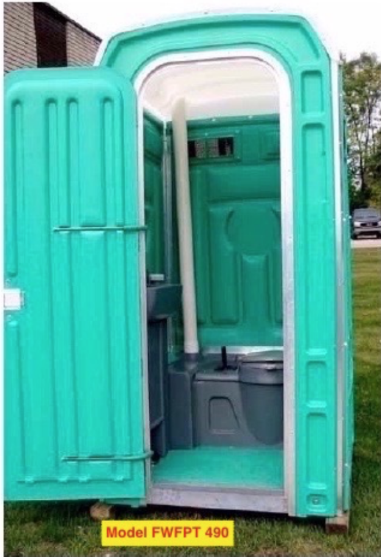
Model FWFPT 490 Has 12 gallon (36 Liter) Water Reservoir Water Reservoir is for Fresh Water Hand Washing and Toilet Flushing
