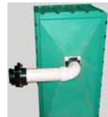
Fig. 3 - Attach Dump Valve
